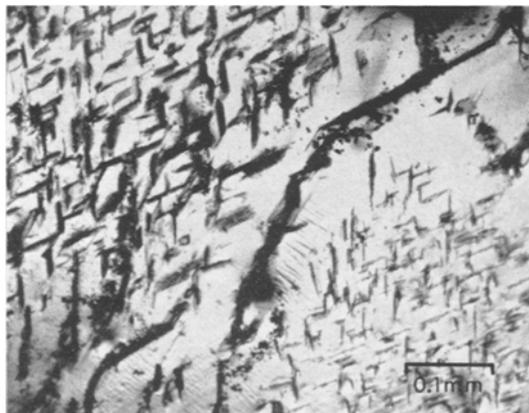
Figure 2 Transmission optical micrograph of a thin section of a natural crystal of MnO containing lathe-like precipitates and voids.
